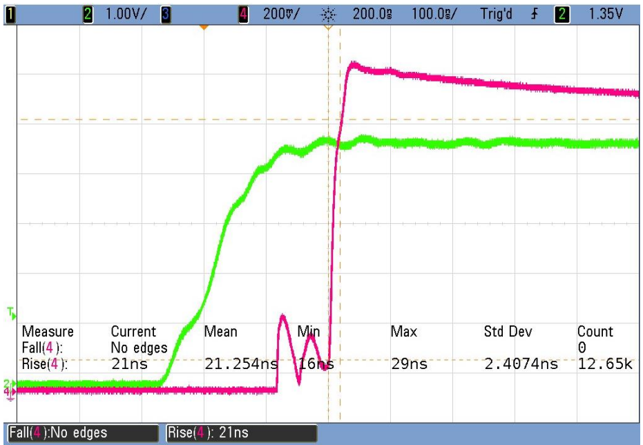
Figure 5: ERZ-HPA-0790-0840-46 Switch ON Time
