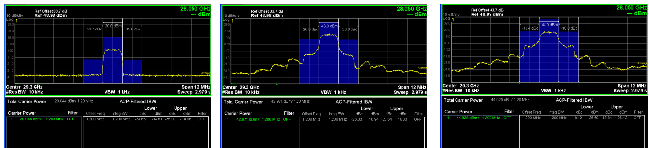
Figure 7: Right—ACPR for BPSK @ 45 dBm output
