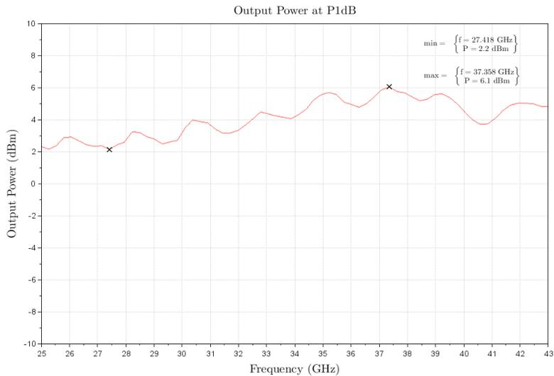
Figure 1: ERZ-LNA-2500-4300-33-2 P1dB
