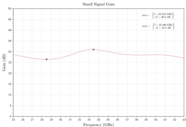
Figure 2: ERZ-LNA-2500-4300-33-2 Small Signal Gain
