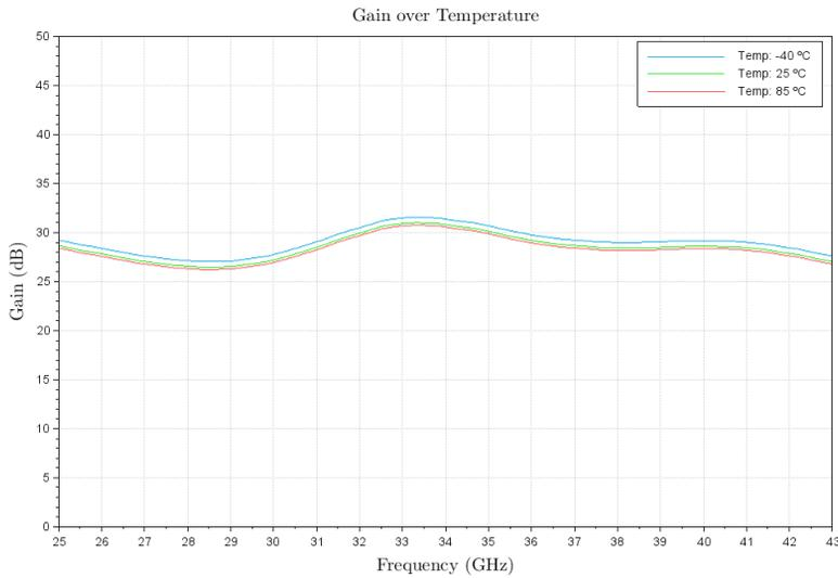
Figure 3: ERZ-LNA-2500-4300-33-2 Small Signal Gain Vs Temperature
