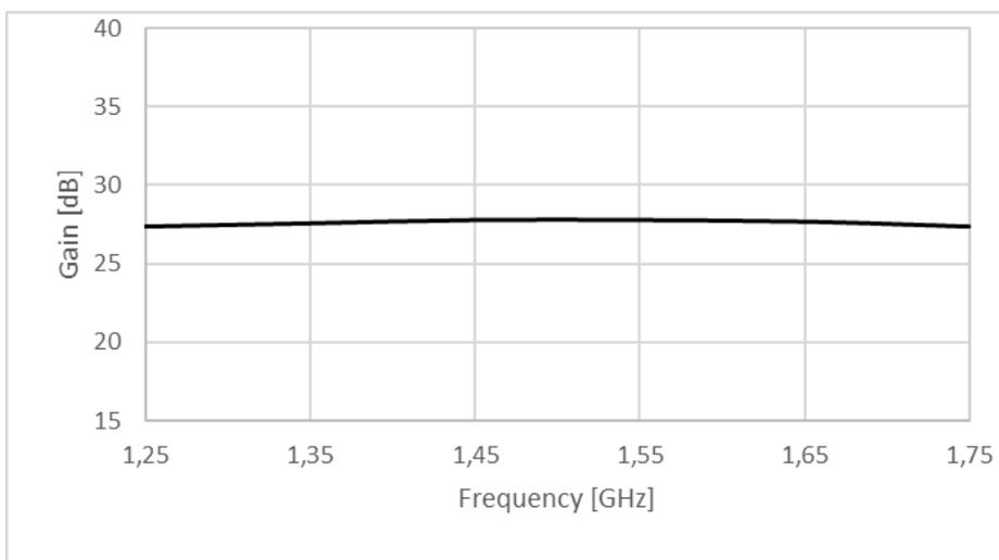
Figure 2: ERZ-LNA-0125-0175-27-2 Small Signal Gain
