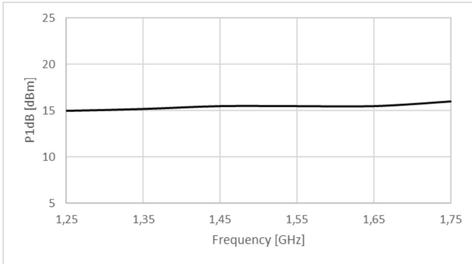
Figure 1: ERZ-LNA-0125-0175-27-2 P1dB
