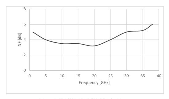
Figure 2: ERZ-LNA-0100-3800-12-4 Noise Figure
