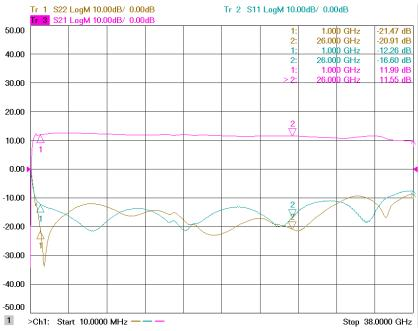
Figure 1: ERZ-LNA-0100-3800-12-4 S-parameters
