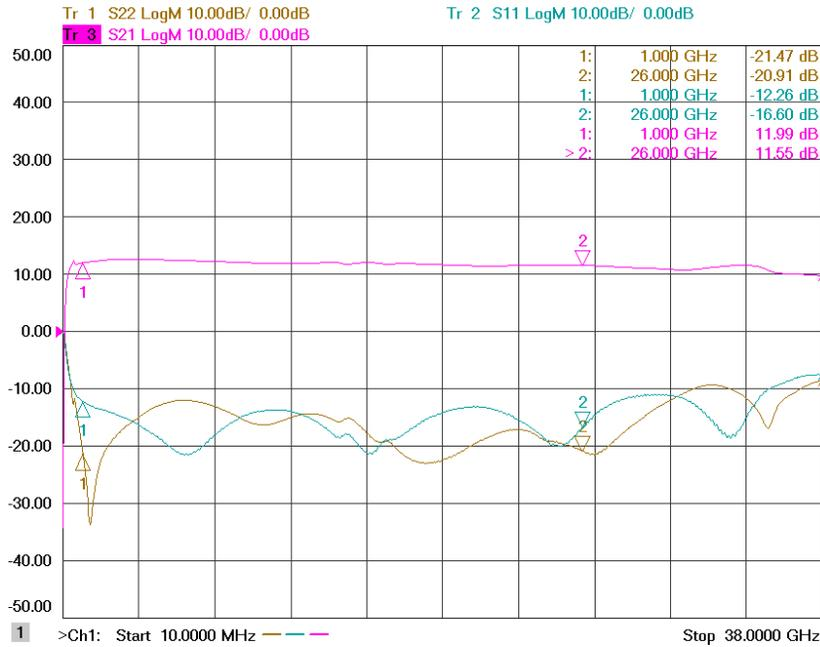
Figure 1: ERZ-LNA-0100-3800-12-4 S-parameters
