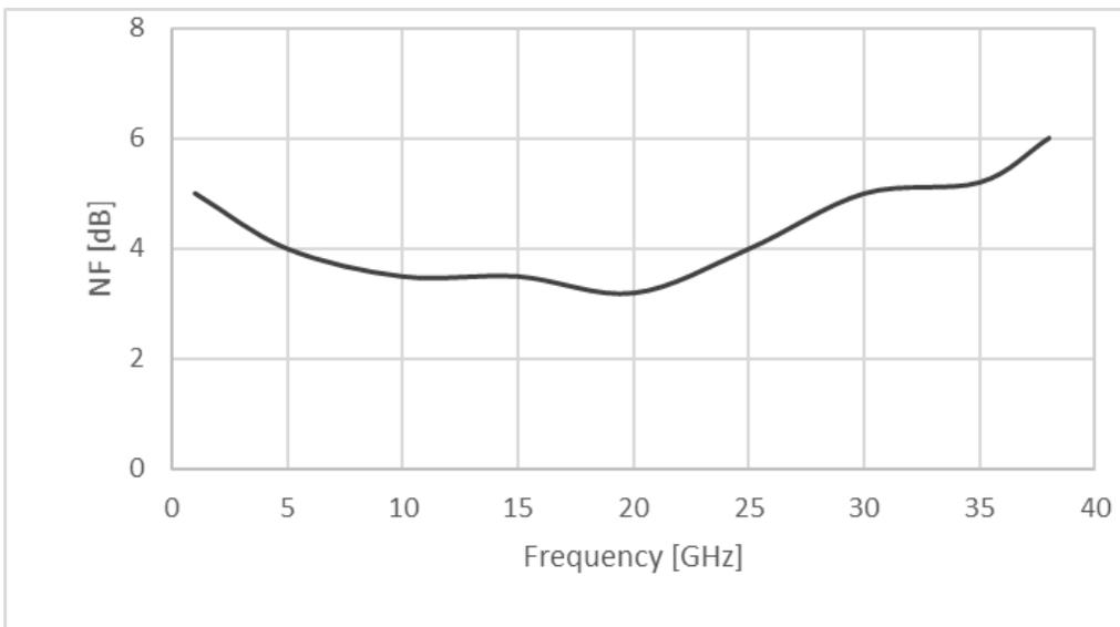
Figure 2: ERZ-LNA-0100-3800-12-4 Noise Figure
