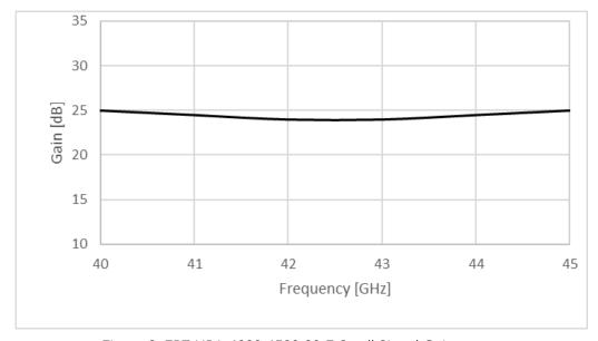
Figure 2: ERZ-HPA-4000-4500-28-E Small Signal Gain
