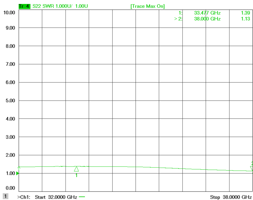
Figure 5: ERZ-HPA-3200-3800-25 Output Matching
