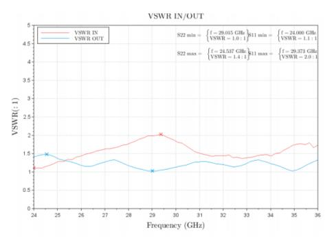
Figure 4: ERZ-HPA-2400-3600-27 Input&Output Matching
