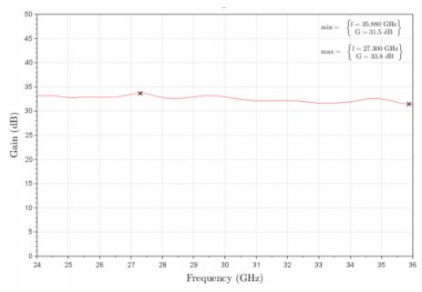
Figure 2: ERZ-HPA-2400-3600-27 Small Signal Gain
