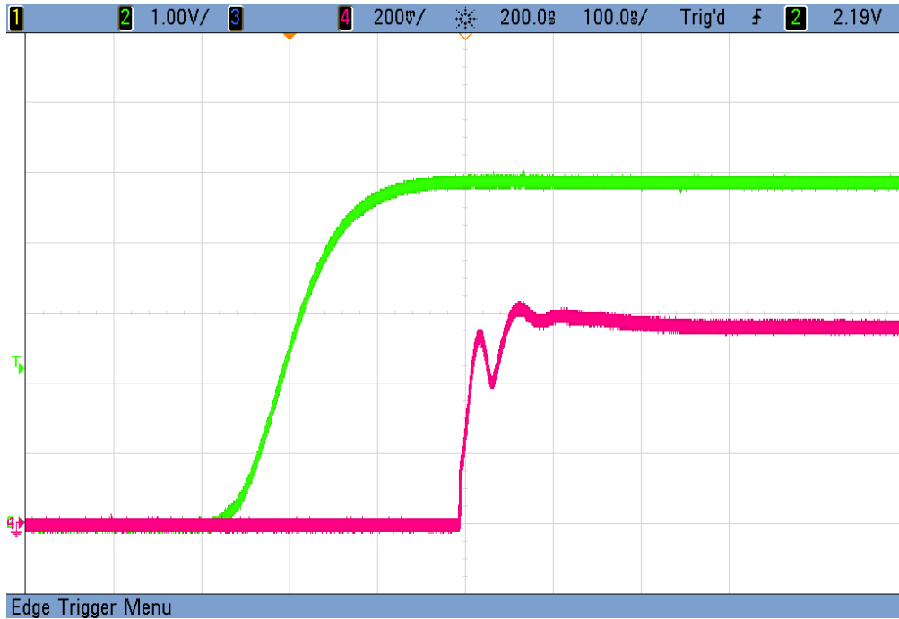
Figure 12: ERZ-HPA-0900-1000-56 Switch ON time
