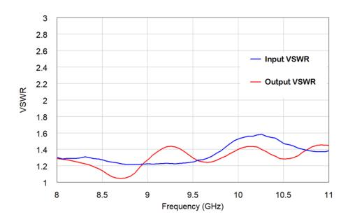
Figure 4: ERZ-HPA-0800-1100-43 Input and Output VSWR
