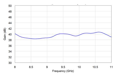
Figure 2: ERZ-HPA-0800-1100-43 Small Signal Gain
