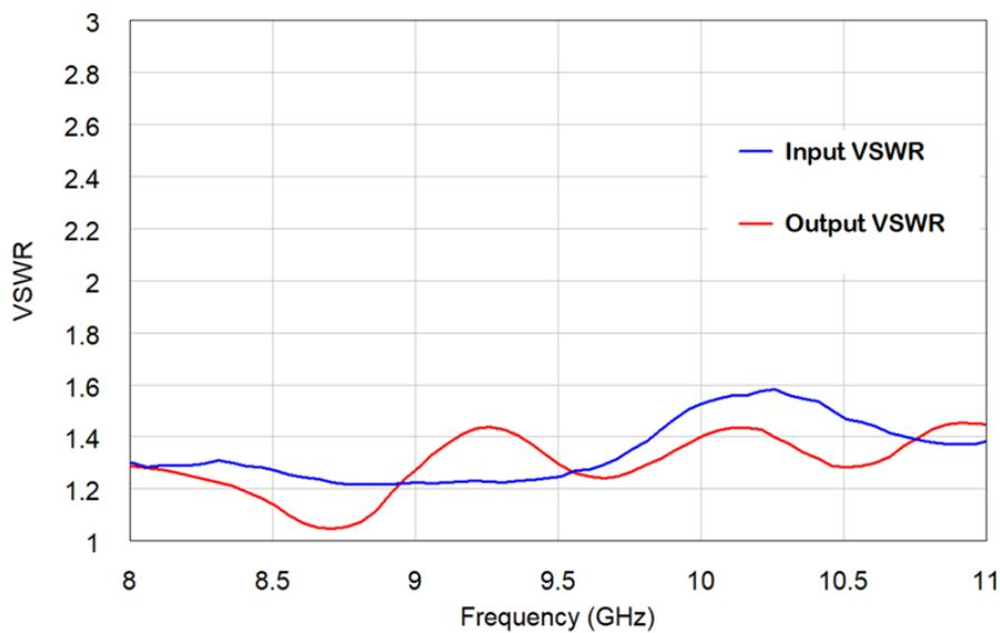
Figure 4: ERZ-HPA-0800-1100-43 Input and Output VSWR
