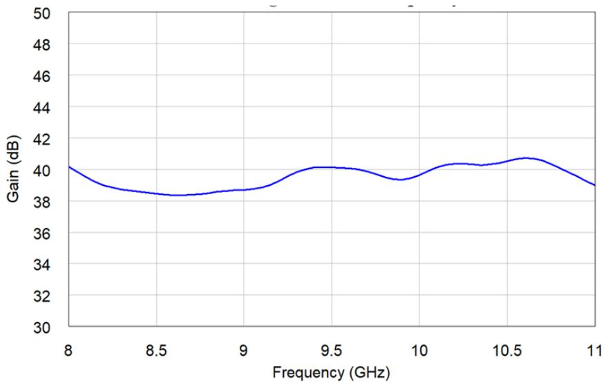
Figure 2: ERZ-HPA-0800-1100-43 Small Signal Gain
