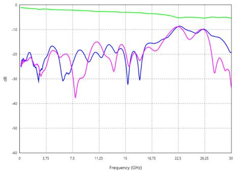
Isolation between not connected ports
