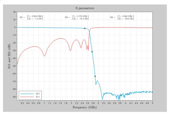
Figure 1:ERZ-LPF-0000-0250-1.3 Insertion & Return Loss
