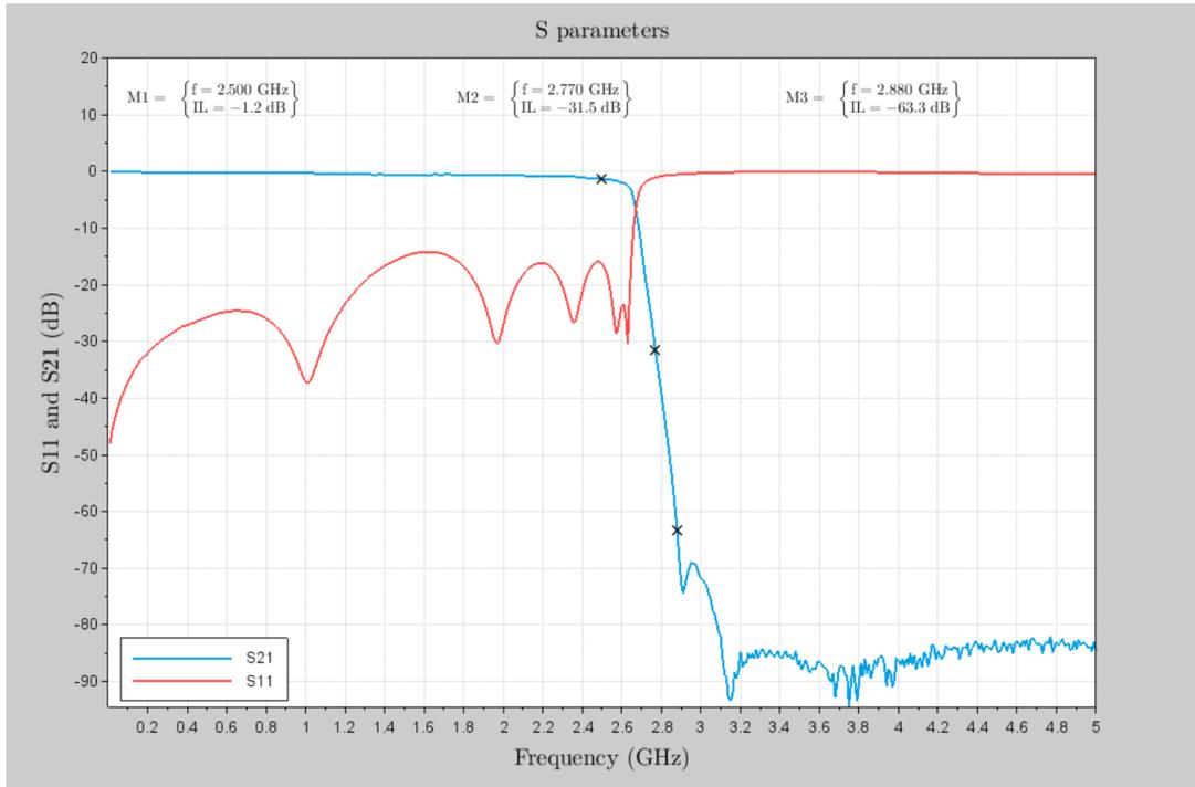
Figure 1:ERZ-LPF-0000-0250-1.3 Insertion & Return Loss
