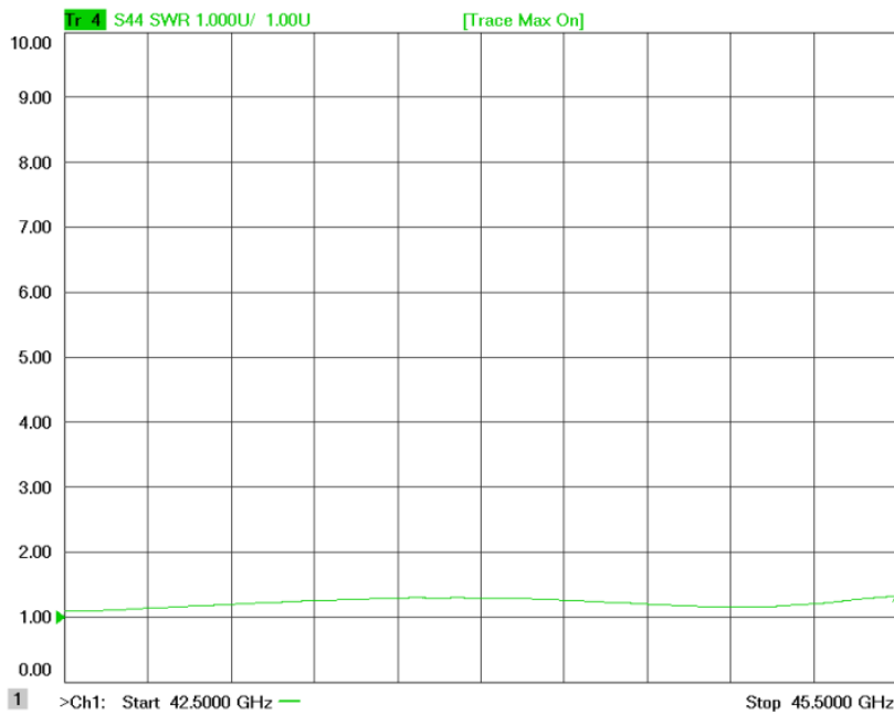
Figure 6: ERZ-LNA-4250-4550-30-4.5 Output Matching
