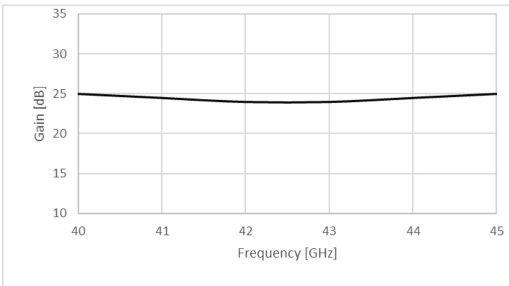
Figure 2: ERZ-HPA-4000-4500-28-E Small Signal Gain
